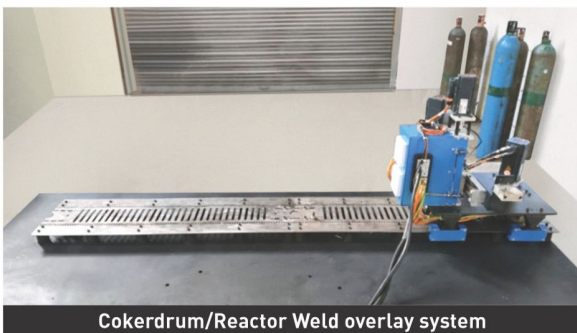
Cokerdrum/Reactor Weld overlay system
