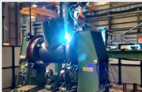
Robotic Welder for Boiler T Joints
