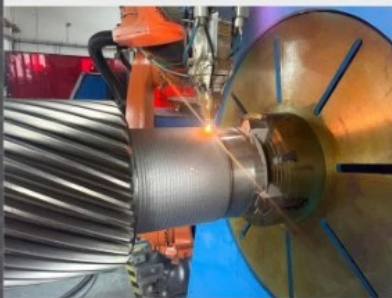
Robotic Laser Cladding
